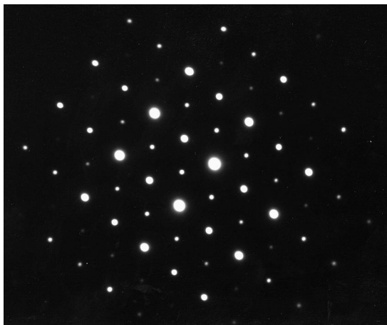
Figure 3 Selected area diffraction pattern with a beam direction of [110]_{L21/A2} showing the cube-cube orientation relationship of the A2 type \alpha -Cr precipitate and L2 1 type Ni 2 AlTi joint centre-line matrix of a sample post-bond heat-treated for 6 h at 1000 °C.
