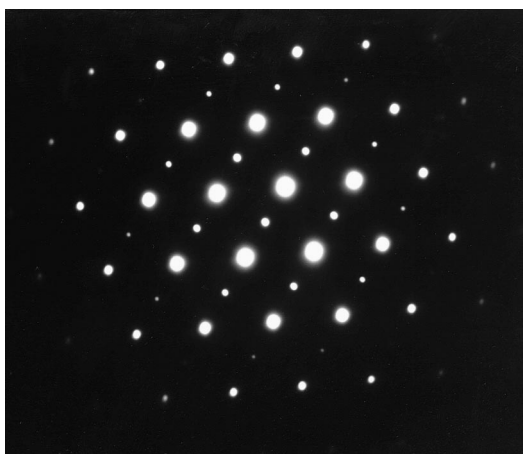
Figure 5 Nano (parallel) beam diffraction pattern with a beam direction of [110]_{L1_2} , taken from an L1_2 type Ni_3(Al, Ti) precipitate in the titanium depleted portion of the NiTi substrate of a joint subjected to a 6 h post-bond heat treatment at 1000^\circ C .
